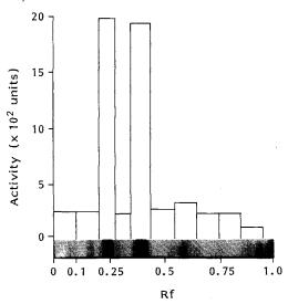
Fraction IV-5 materials were separated on silica gel thin layer plate with solvent and stained as described in Materials and Methods. The materials distributed along the plate were cut out from the unstained plate, eluted and assayed for topo I inhibition. Rf's are shown in the abscissa and inhibitory activities in units in the ordinate.
